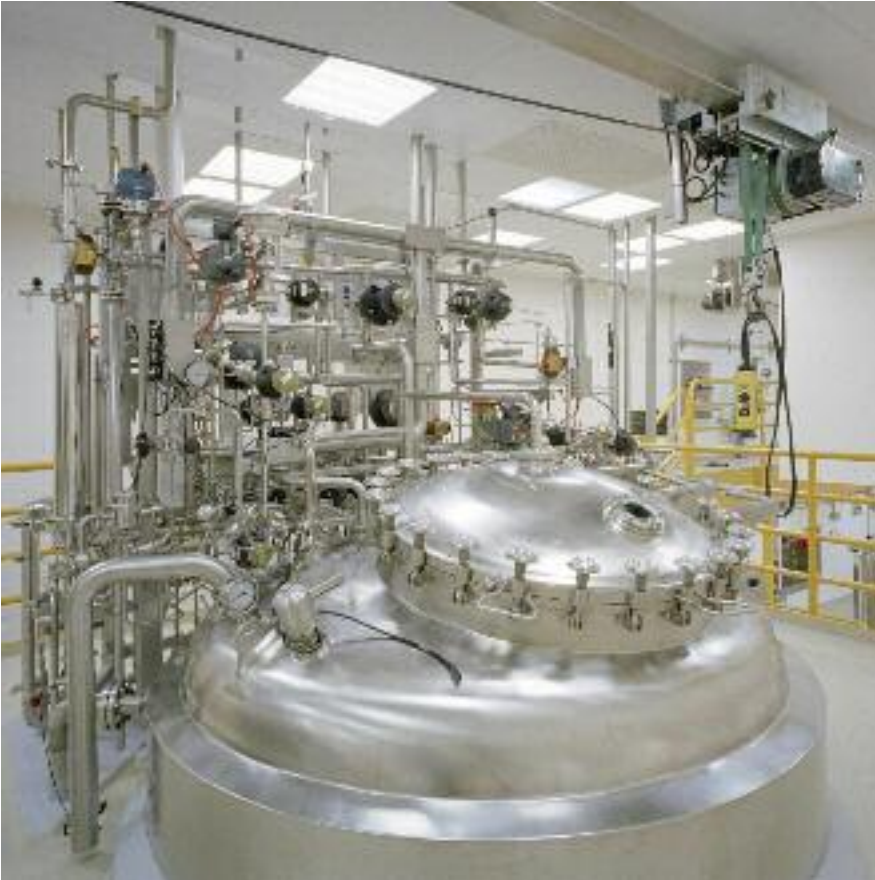
Fed-batch fermentation using animal cells for the production of biopharmaceuticals at one of the ACTIP member companies (Genzyme).
